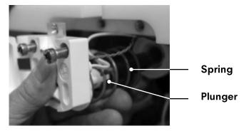
3. Gently remove the valve door, plunger, and spring from the valve body. The metal valve insert and reed switch sensors are wired to the dispenser and are threaded through the valve body. In some cases, the valve body style will prevent it from being completely removed from the dispenser.
