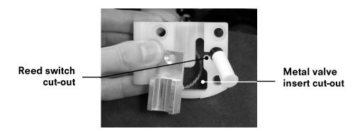
4. Remove the round plastic ring (spring retainer) from the solenoid. It cannot be fully removed from the dispenser as the metal valve insert and the reed switch wires are threaded through an eyelet on the plastic ring (spring retainer).
