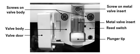
Firmly hold the valve body assembly (the spring may push the valve assembly forward when removing the screws). Remove the two screws from the upper corners of the valve body. Set aside the screws for cleaning.
